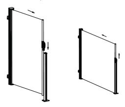
2. When you want to close it, hold the handle and pull up the handle spindle. Keeping the fabric horizontal and push the handle back to the cover slowly.
