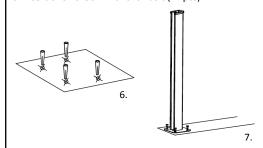
7. Make the left bottom hole of stand fix and the hole on the floor alignment and tighten them with M8x75mm hexagon wooden screw.
